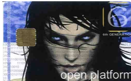
Figure 2.2: Sample picture of a Funcard with an AVR microcontroller
